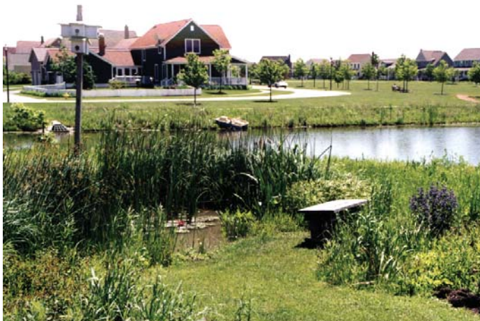
Rain gardens capture and cleanse rooftop runoff and provide wildlife habitat and aesthetics.
