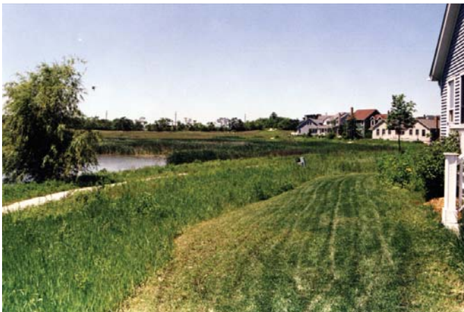
Natural buffers between homes and detention basins filter pollutants from stormwater runoff.
